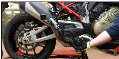
**ENG** Undo the fastening screw and remove the heat guard
